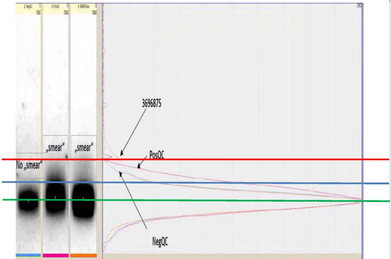
Figure 5: The same as the figure on previous page but with expanded vertical axis in order to more clearly see the differences between the three profiles. Moreover, the figure includes horizontal lines that indicate where the peak due to eEPO appears (green horizontal line), where the peak due to rEPO is expected (blue horizontal line) and where the peak that contributes to the «shoulder» in the athlete's lane is expected (red horizontal line). Where these peaks are predicted to come (if the positive control and the athlete's sample did not contain eEPO) is estimated by subtracting the negative control profile (NegQC) from, respectively, the positive control profile (PosQC) and the athlete's profile. It is assumed that the three samples contain similar amounts of eEPO, which should not be a "way-off" assumption since these profiles have been normalised/standardised so that their maximum heights/intensity (which is mainly due to eEPO) is identical. The conclusion that the athlete's "shoulder peak" migrates more slowly than rEPO and thus does not coincide with rEPO in the positive control is evident in all subsequent profiles the laboratory presents upon testing the B-sample.
